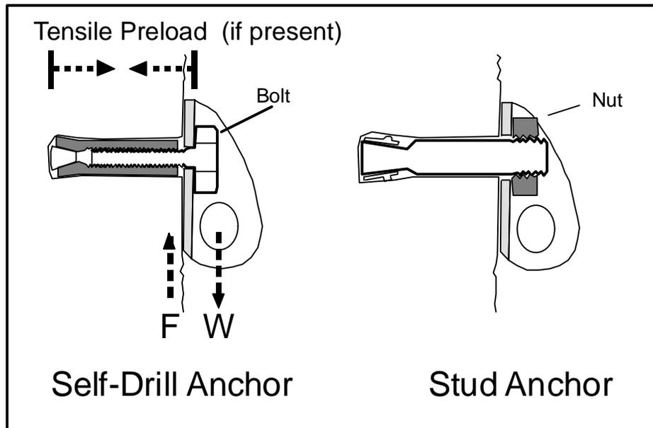
Figure 2: Idealized self-drill and stud anchors in tight holes. Axial preload enables the rock/hanger interface to oppose the load applied by the rope ( $W$ ), with friction force ( $F$ ). Note that the self-drill anchor is optimally placed just below the rock surface.
