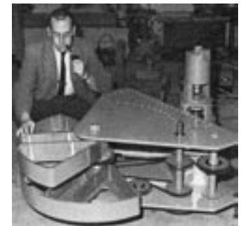
In 1959, Caughey designed a portable earthquake-making machine, a.k.a. an eccentric-mass vibration generator that was the forerunner of the shaking machines used by civil engineers around the world today.
