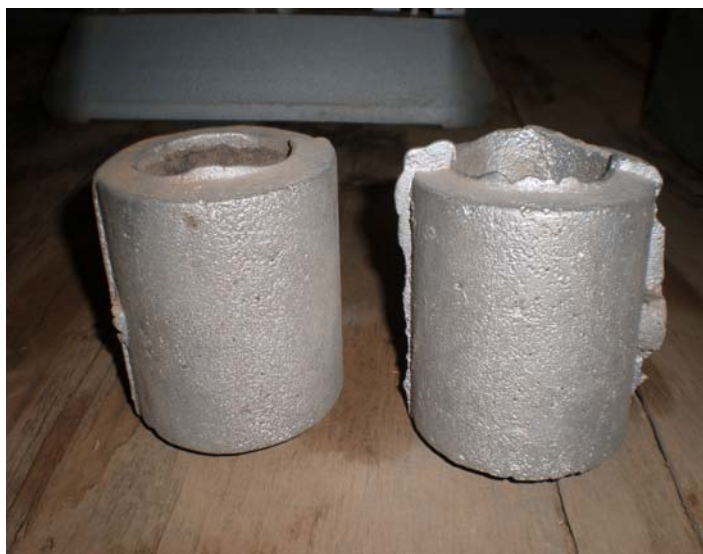
Plate 1. Test Castings Produced from Aluminium Alloy using Yola Natural Sand
